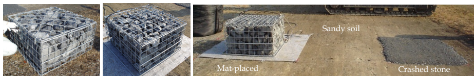
(a) Diamond-shaped (b) Grid-shaped (c) Ground surface condition to place gabions
